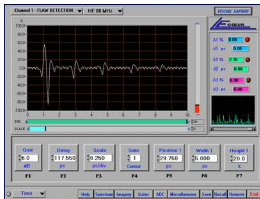
Figure 4b. Response on 1.6mm aluminium skin
